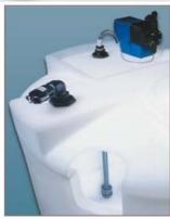
Assmann Corporation advises that using its Double Wall Tank system with a bottom sidewall fitting may not meet local codes for secondary containment, as tank contents could escape containment area in the event of fitting damage. Assmann recommends that its Double Wall Tanks be fitted with a top suction line and foot valve to provide constant flow to the pump.
